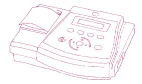
The portable, battery powered "Mac 400" ECG by General Electric costs less than half the price of a conventional device. Treating a patient costs just one dollar rather than the usual ten. It has only four buttons, and the printer is the same model used on buses to print tickets. Developed for undersupplied rural areas in India, the device has also been a big hit worldwide.
