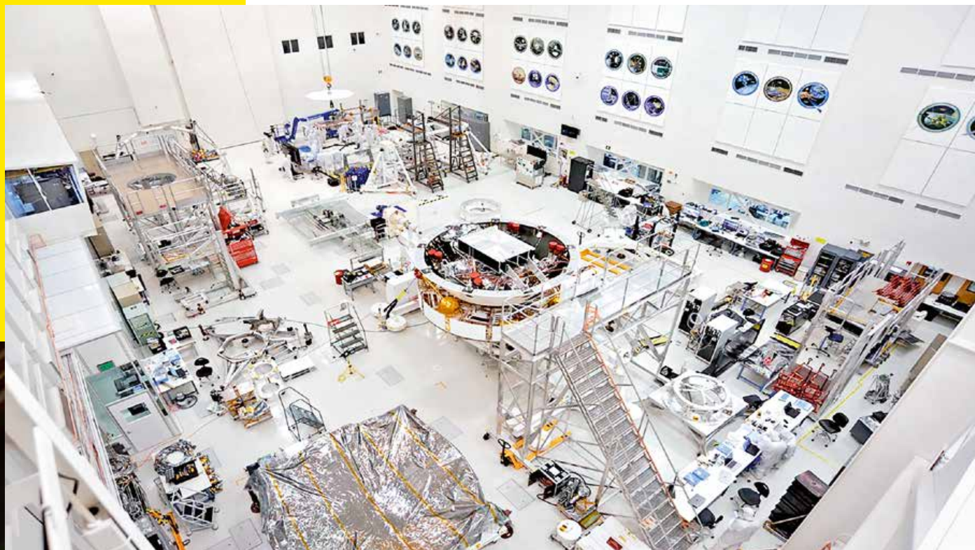
CLEAN RESULTS Assembly of the rover and its components takes place in a clean room to ensure any samples that may return to Earth are not contaminated.
