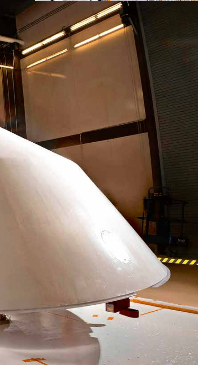
CLEAN RESULTS Assembly of the rover and its components takes place in a clean room to ensure any samples that may return to Earth are not contaminated.
