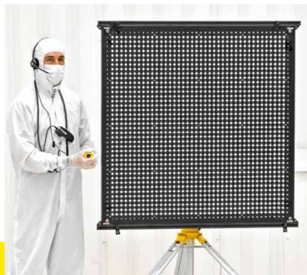
ON THE DOT The forward-facing cameras were calibrated using target boards, a machine vision "eye" exam.
