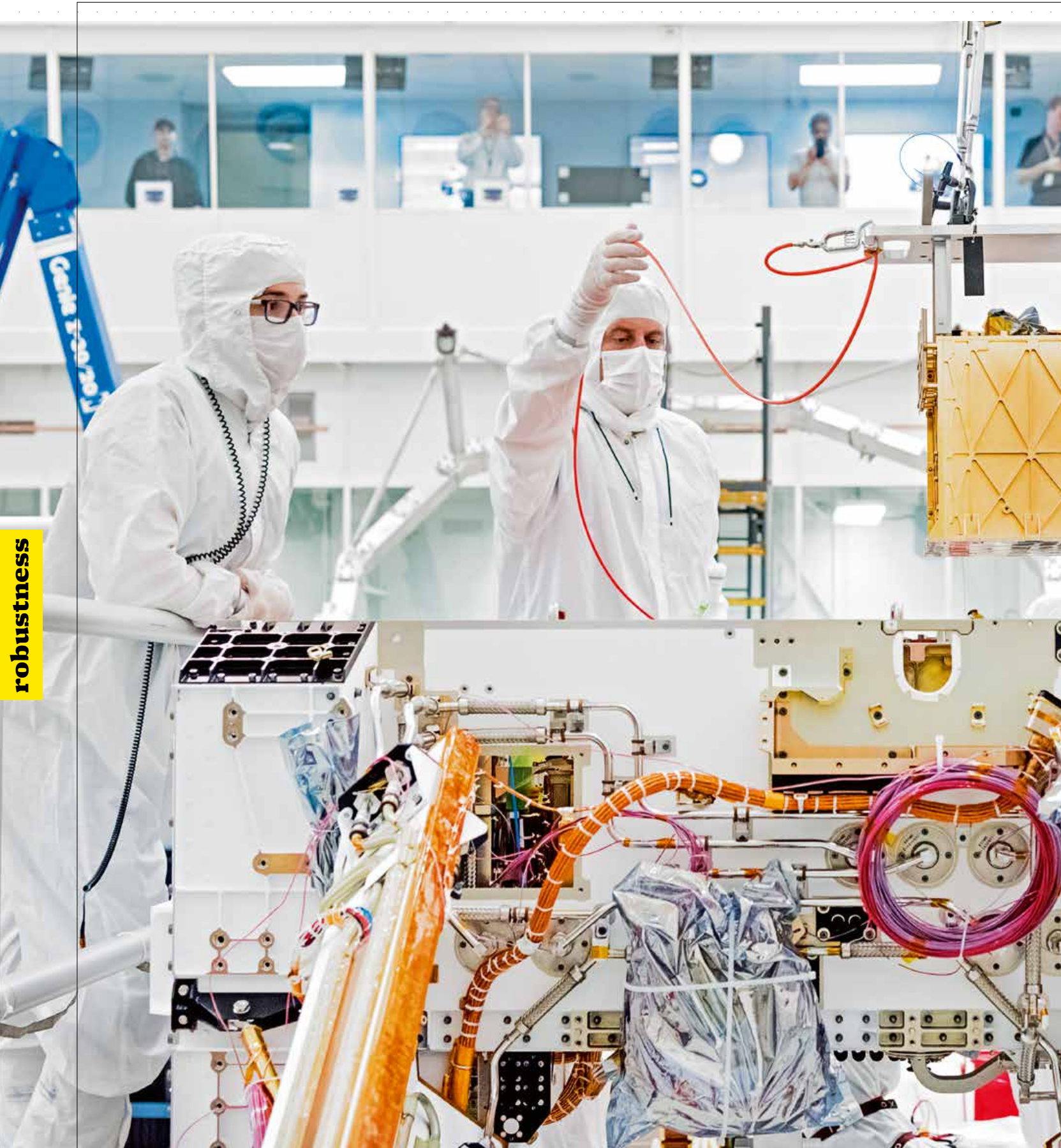
OUT OF THIN AIR The Mars Oxygen In-Situ Resource Utilization Experiment (MOXIE) unit will demonstrate if future explorers can produce oxygen from the Martian atmosphere.
